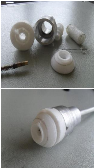
Figure 1. Components of plasma needle (left) and plasma needle (right).
