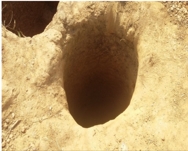
Photo I: Ore extraction well (Alihamdoullilae).
