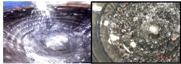
Picture(1): Experiment with three vortex breaker shaft spillway
