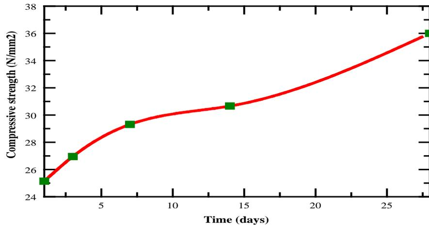
Fig. 6: Compressive strength with relation to time
