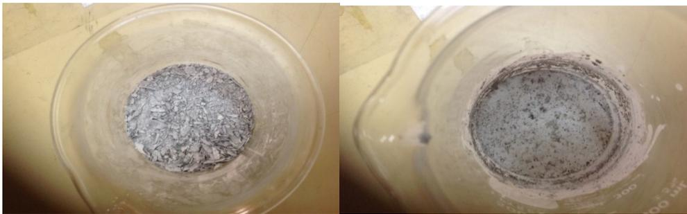
**Fig. 4a: Sample of locust bean pod ash & powdered calcium hydroxide**
