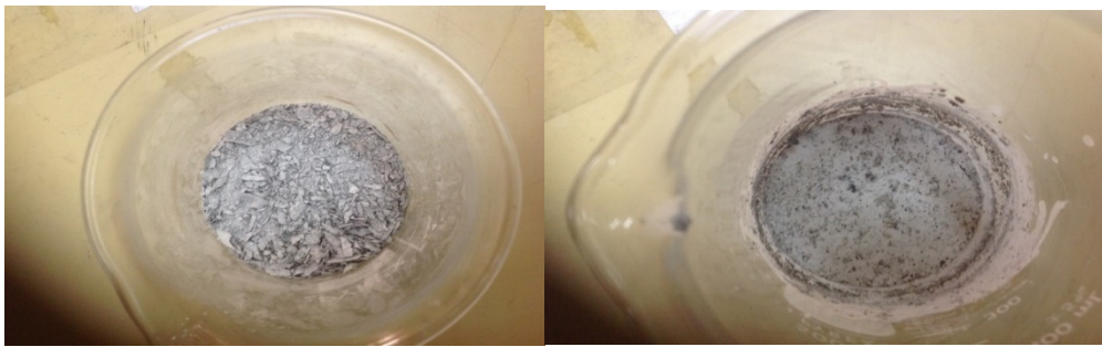
Fig. 4a: Sample of locust bean pod ash & powdered calcium hydroxide Fig. 4b: Dried sample of mixture
