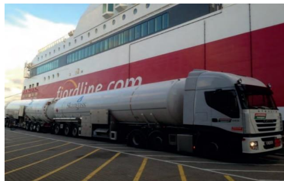
Figure 4. Refueling by truck-to-ship transmission system using two LNG carriers (Skangass Norway refueling station)
