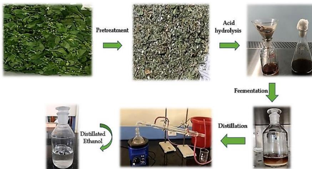
Figure 3. Schematic representation of the bioethanol process
