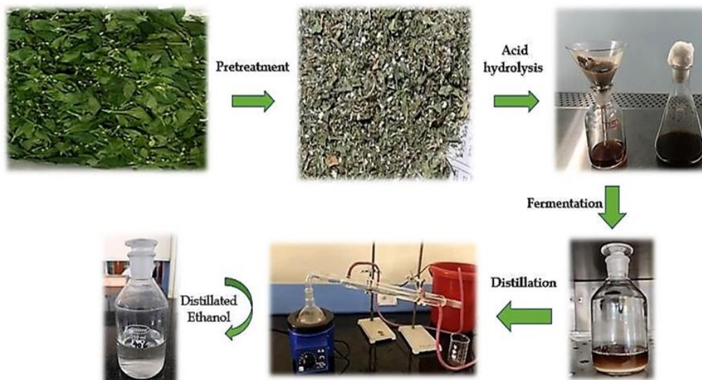
Figure 3. Schematic representation of the bioethanol process
